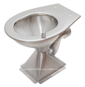
DESICRIPFranke Model HCL Pedestal WC Pan, unit to be manufactured from Grade 304 (18/10) Stainless Steel, 1,2mm gauge. Unit to be manufactured with a pressed flushing rim and integral "P" Trap with a 102mm outlet pipe, and a 60mm back entry inlet pipe to suit a rubber flush inlet sealing bung. The pan to be fitted with a Stainless Steel base which has flanges with 6mm holes for fixing the pan to the floor (bolts elsewhere measured).TIONS
